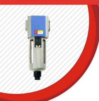
Offers Automatic industrial lined filters. These filters have low pressure loss, high efficiency in separating water and large drain bowl capacity. It can effectively separate liquid from air and filter solid particles reliably. Filtering grade includes 5 µm and 40 µm. Three drain types are available: manual drain, semi-auto drain and automatic drain.
