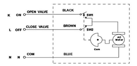
1.Connecting SW1 and OPEN, the valve opens, getting the position, automatically power off, the valve remain fully open position.
