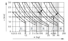
Three force curves are shown for each shock absorber. An average must be taken for intermediate values.
