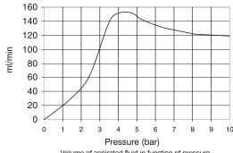
Volume of aspirated fluid in function of pressure power with the adjuster screw "V" totally open
